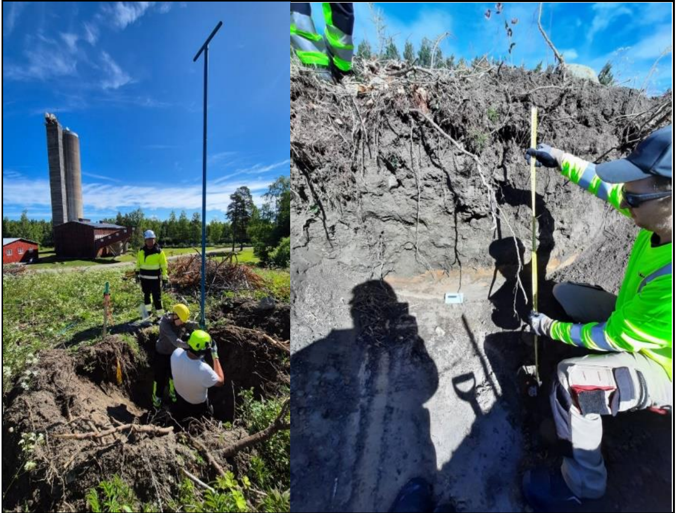
Figure 2: Post removal of a barren rock cap samples can be extract with no wall contamination down to basement at 7.5m depth.
